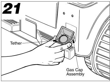
Snap the gas cap assembly into the square opening in the rear of the vehicle. (The gas cap tether should point down.)
